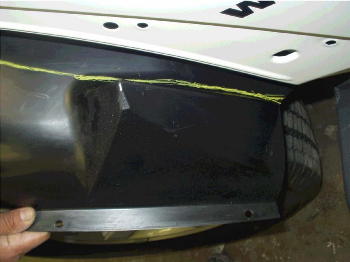
This picture shows a portion of the front liner marked for trimming. The liner has been pulled out several inches to illustrate the grease pencil trim mark. This view is from the top of the liner looking toward the rearward section of the liner.
