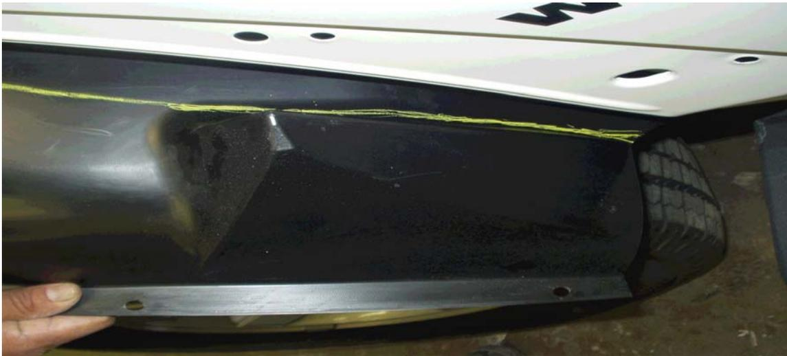
**Figure #1-** This picture shows a portion of the front liner marked for trimming. The liner has been pulled out several inches to illustrate the grease pencil trim mark. This view is from the top of the liner looking toward the rearward section of the liner.
