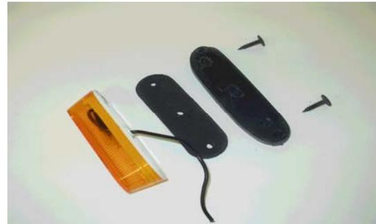
**-LOCATE the aftermarket running lights, the wire connectors, the Xenon urethane oval shaped backer plates (has 5 holes in it), the silver Phillips screws and #8 screws from the hardware package. This will be the hardware you need for the front flares to install the side marker light that fits our part.**
