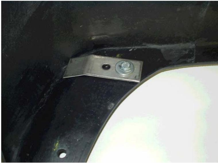
**-BOLT** the flares to the body at 9 points using the 1/4"-20 x 3/4" bolts, 3/4" fender washers (one on the bolt head side and one on the inside of the steel body) and the 1/4-20 nylon lock nut. Do not over-torque (10 foot/pounds). On the #2 hole from the front, before bolting up, attach the angled steel bracket outside our part flange and secure with the bolt, nut and washers.
